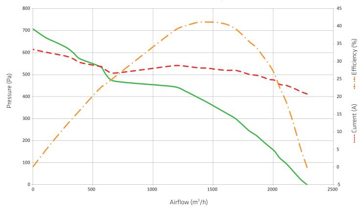
Pressure: 1Pa=0.004 inH₂0 Airflow: 1m³/h=0.59 cfm
