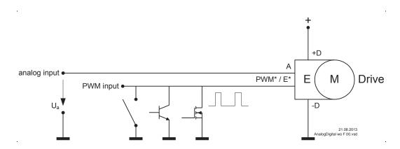
In this operating mode the supply voltage plus is usually connected permanently. To run the Drive on the pin PWM $^*$  / E $^*$  a PWM signal has to be applied and with the duty cycle of the PWM signal the Drive speed can be then controlled. If the pin PWM $^*$  / E $^*$  is switched to supply voltage minus the Drive speed can be then controlled with an analog voltage on the pin A.
